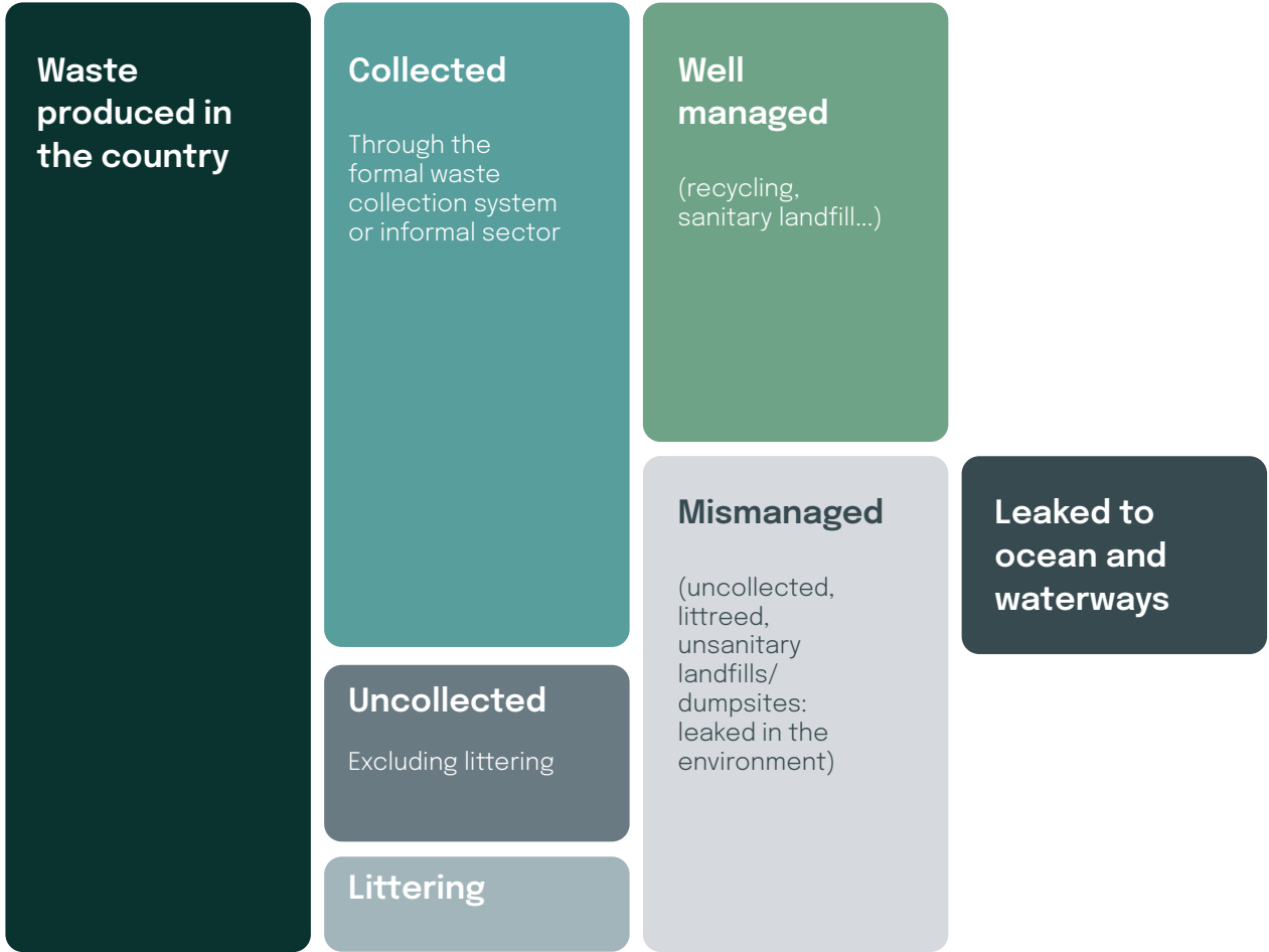
Fig. 5. The diagram shows the plastic flow, from waste production to leakage.
