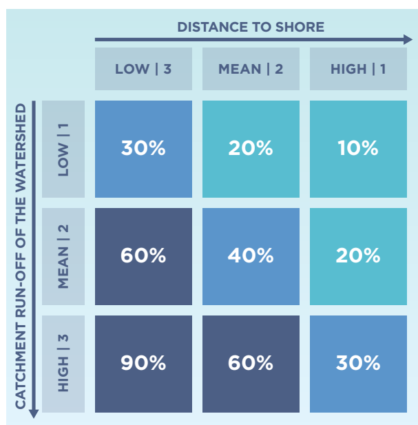
Figure 13: Release rates matrix for country assessment. Distance classes are 10km (low), between 10 and 50 km (mean), and above 50km (high). Run-off categories are <0.4 \text{ mm.day}^{-1} \text{ km} (low), between 0.4 and 0.8 \text{mm.day}^{-1} (mean), and >0.8 \text{ mm.day}^{-1} (high).
